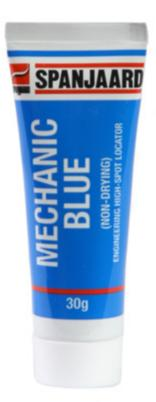
Engineering high-spot locator is a blue paste for locating high-spots on mating surfaces such as bearings and shafts. High-spots will be shown as bright streaks when shaft is turned in the bearing.
